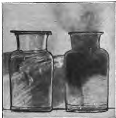
FIG. 59.—The colorless nitric oxid unites with oxygen to form the reddish-brown nitrogen peroxid.
